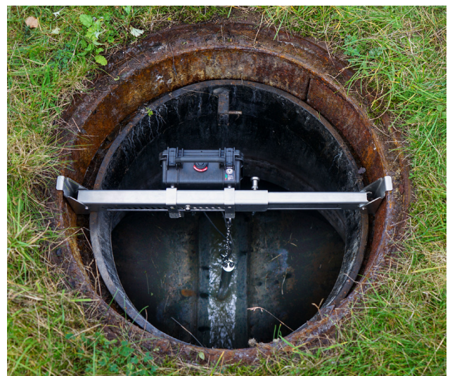
Figure 5 - Example of a liquid-phase H_2S sensor.
