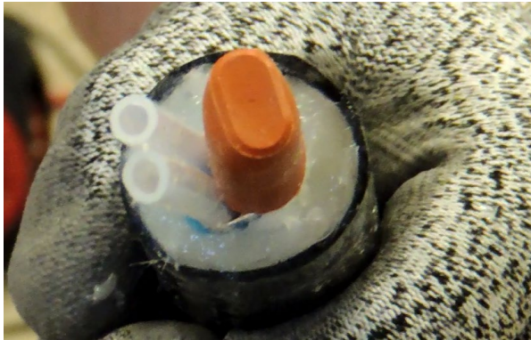
Figure 8 Heated sample line, HSL to be connected to probe
