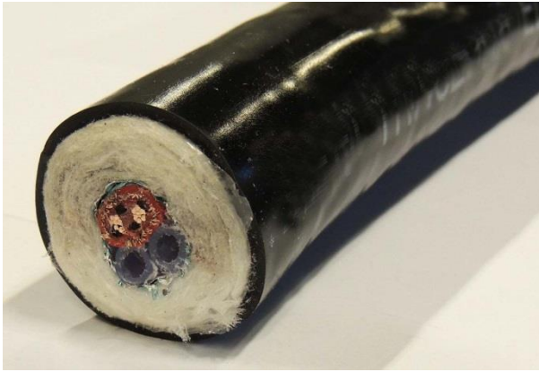
Figure 13 Heated sample line as delivered
