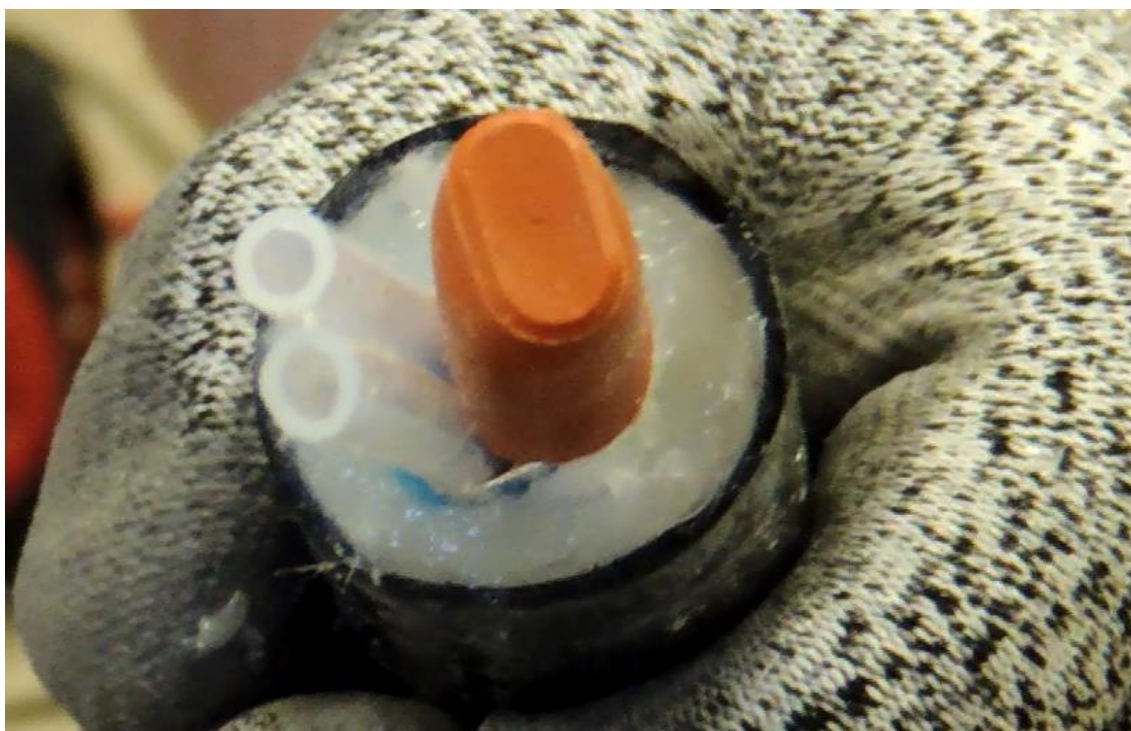
Figure 7 Heated sample line to be connected to probe (and one spare)
