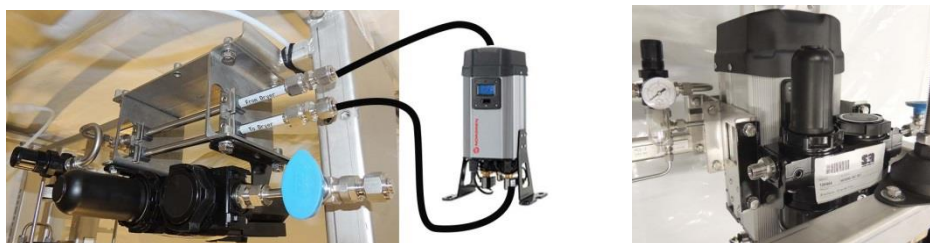
Figure 30 Compressed air dryer. External mount (left) and internal mount (right).
