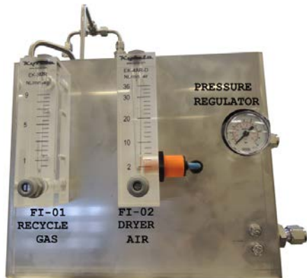
Figure 8 Flowmeters and regulator on SCS
