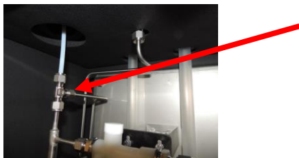
Figure 7 T-piece in the SCS cabinet
