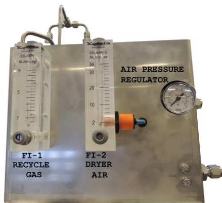
Figure 8 Flowmeters and regulator on SCS
