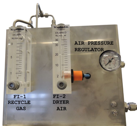
Figure 8 Flowmeters and regulator on SCS
